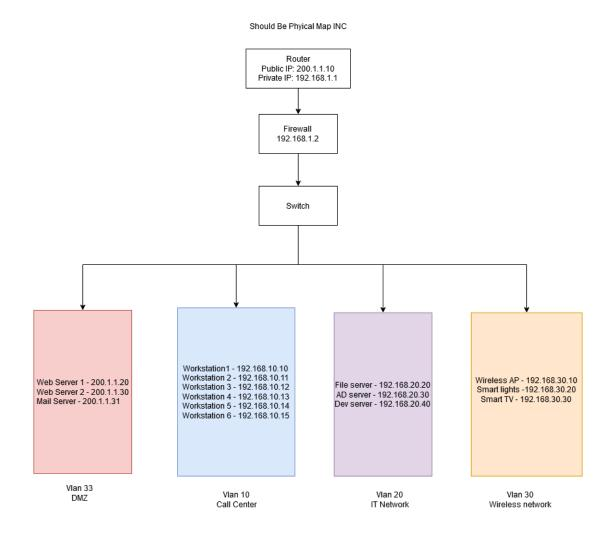
The original logical map included a router, firewall, and switch, with 4 VLANs, for the DMZ, Call Center, IT Network, and Wireless Network. Each device was assigned an IP address,
